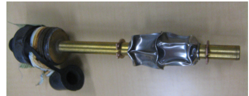
Crushed Float Sensor
